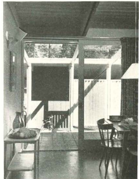
Opposite view from upper left photo. This shows how vertical louvers on the carport create a baffle from light, shutting out sight of automobile and creating a more screened entrance. Open roof framing beyond door ties dining and garage together yet lets in light.
