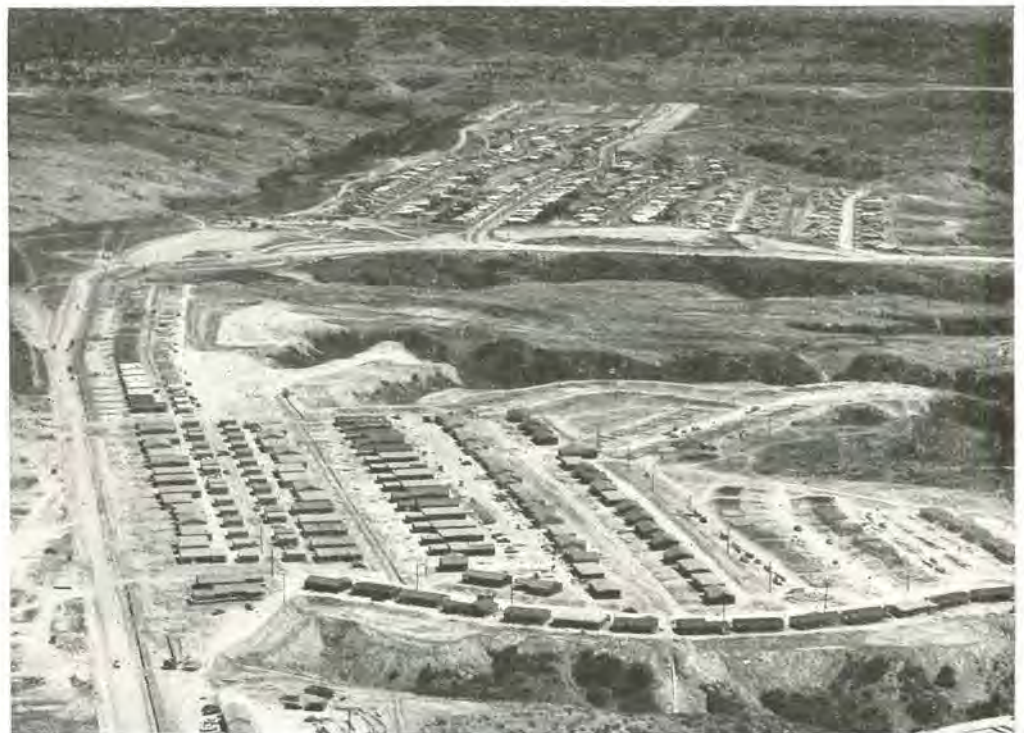
BIGGEST DEFENSE HOUSING development is Clairemont, where Burgener-Tavares and four other combines plan to erect 4,322 units. The steep gullies facing the 3,000 acre site are typical of the treeless mesa land at the north edge of San Diego where much defense housing is located. For their project, Burgener-Tavares had to build a mile of sewer main to connect with city lines.
